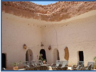
Figure 4: Sloped terrain and soft rock in Ghiryan, Libya, enabled traditional underground atrium houses. Source: (Photo Researcher)
